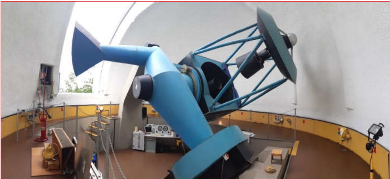
Figure 2 – A panoramic view of the “G.D. Cassini” telescope at the Loiano Observatory in its original configuration. In operation since year 1975, the telescope has a Ritchey-Chretien optical design and sports an f/3 primary mirror of 152 cm in diameter. An equivalent focal ratio f/8 is reached at the Cassegrain focus, currently equipped with the BFOSC CCD camera.
