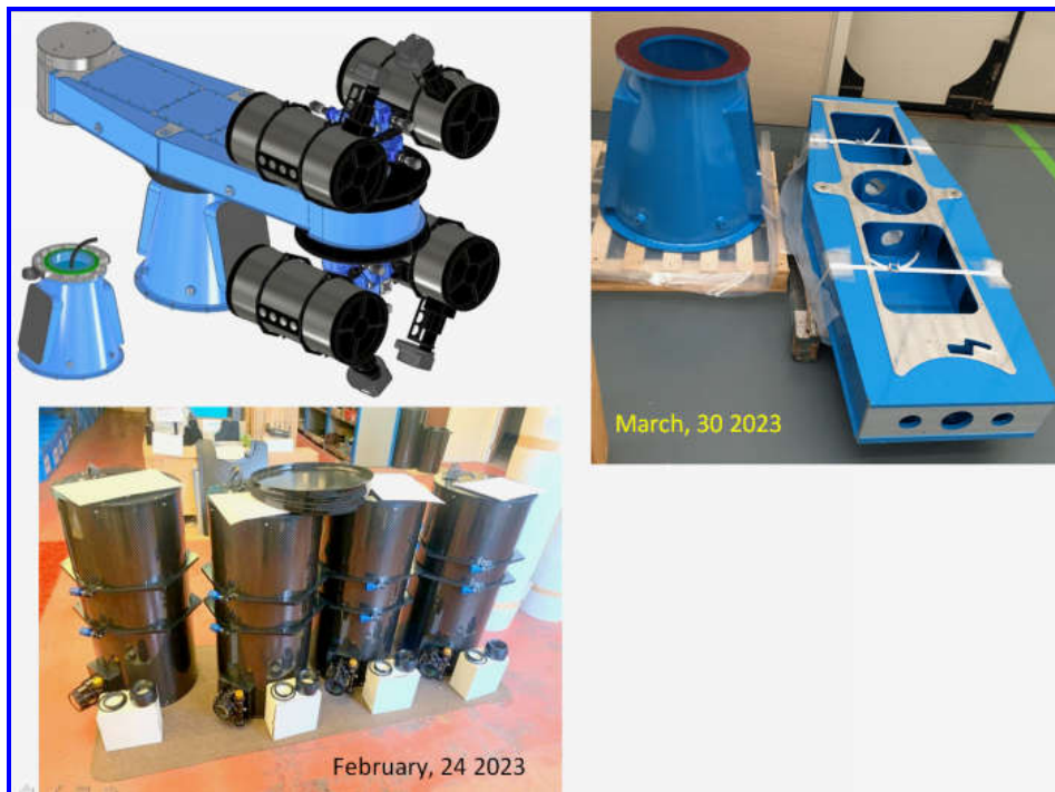
Figure 6 – A few milestones along TANDEM assembly. As a reference, top left is the final concept of the instrument, which began to take shape in spring 2023 with the acquisition of the four ORION telescopes (bottom left) and the manufacturing of the steering arm (top right) with the conic flange to anchor the instrument to the Cassini mount.
