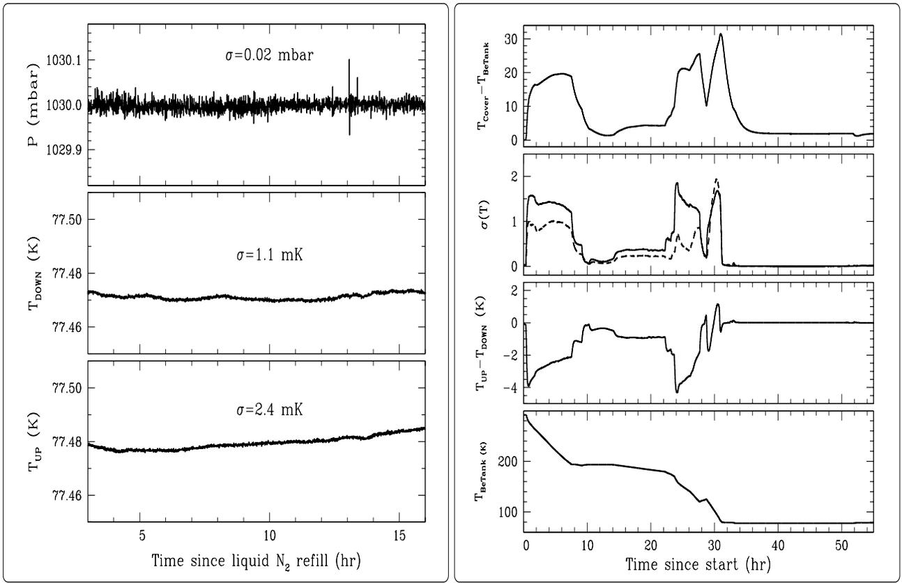
**Figure 1.** Left hand panel: variation of N<sub>2</sub> out-boiling pressure and BeTank temperature as a function of time since last refill, see Sect. 2 for details.
