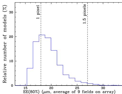
**Figure 2.** Predicted optical quality of the GIANO spectrometer achievable with the alignment procedure described in Sect. 3. The histogram is the distribution from 5,000 models with randomly distributed starting configurations. See Sect. 3 for details.
