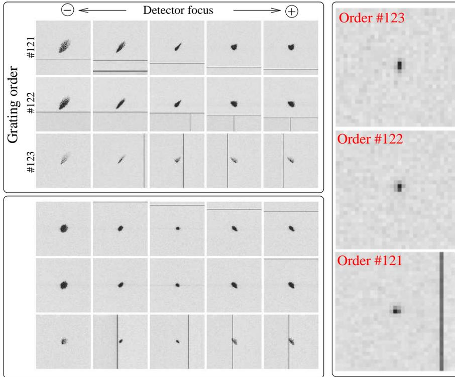
**Figure 3.** Left panels: intro and extra focal images during various phases of the alignment of GIANO with the HeNe 633 nm laser. The dark stripes are intrinsic defects of the Hawaii-II multiplexer. Right hand panel: zoomed view of the images when the system is aligned and focused. See Sect. 3.2 for details
