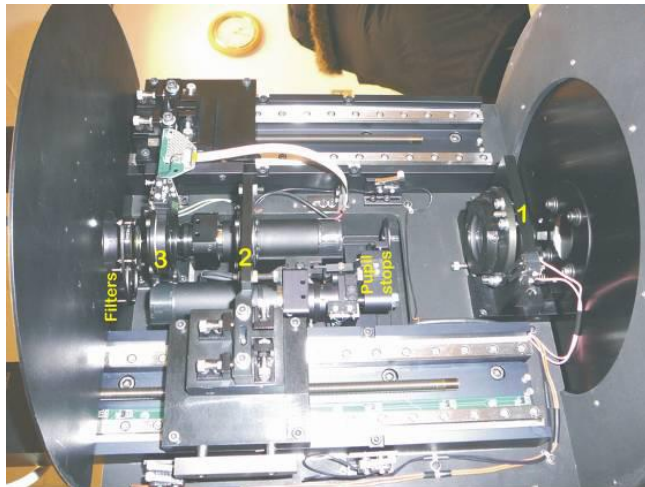
Figure 8 View of the opto-mechanics of the TC number 2.
