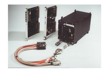
The second generation was introduced in 2005 and was based on the San Diego State University (SDSU) systems deploying DSPs on PCI bus bridged to Motorola PowerPC VME boards and e2v detectors integrated in ESO made camera heads.
