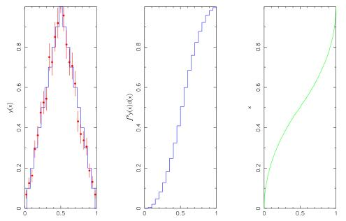
An example of generating a Monte-Carlo distribution following a known histogram. Left: the step-ladder histogram, with points from 2000 trials, produced by a) integrating the function (middle) and b) transforming the axes to produce f<sup>-1</sup> of the integrated distribution (right). The points with  $\int N$  error bars in the left diagram are from drawing 2000 uniformly-distributed random numbers and transforming them according to the right diagram.
