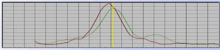
W3OH @ el = 33° with mech. Optical alignment, Tamp = 54K Optics is not aligned properly
