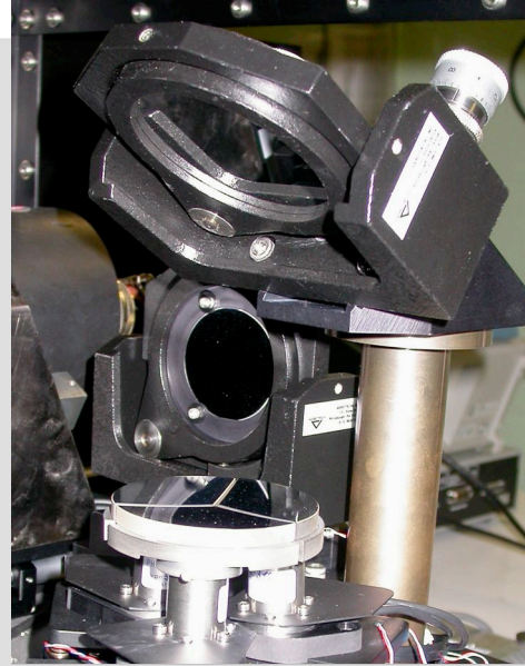
Testbed Mirror with 3 Segments
