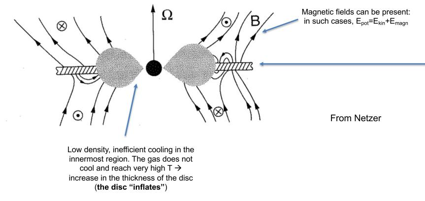
Inefficient conversion of gravitational to radiated electromagnetic energy because most of this is advected ('lost' in the BH) → low resulting luminosities
