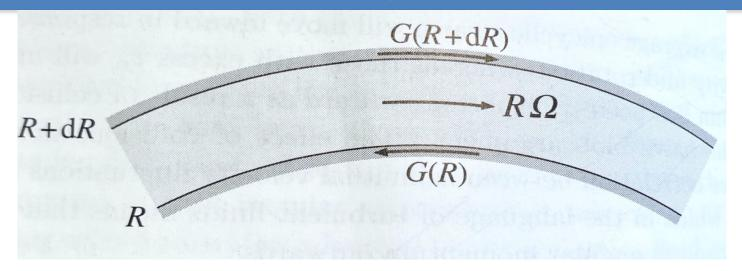
Net torque on a ring of gas between R and R+dR. The ring is subject to competing torques since it has an inner and a outer radius
