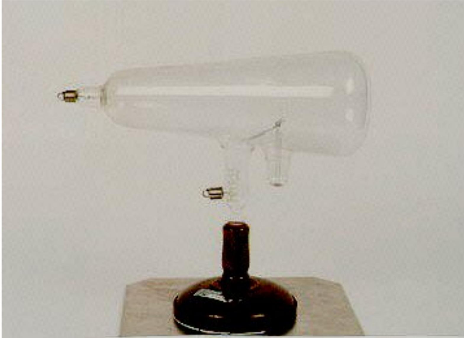
Crookes tube: electrons (produced by high voltage) interact with the walls (glass) and produce fluorescence. Photographic films around are impressed
