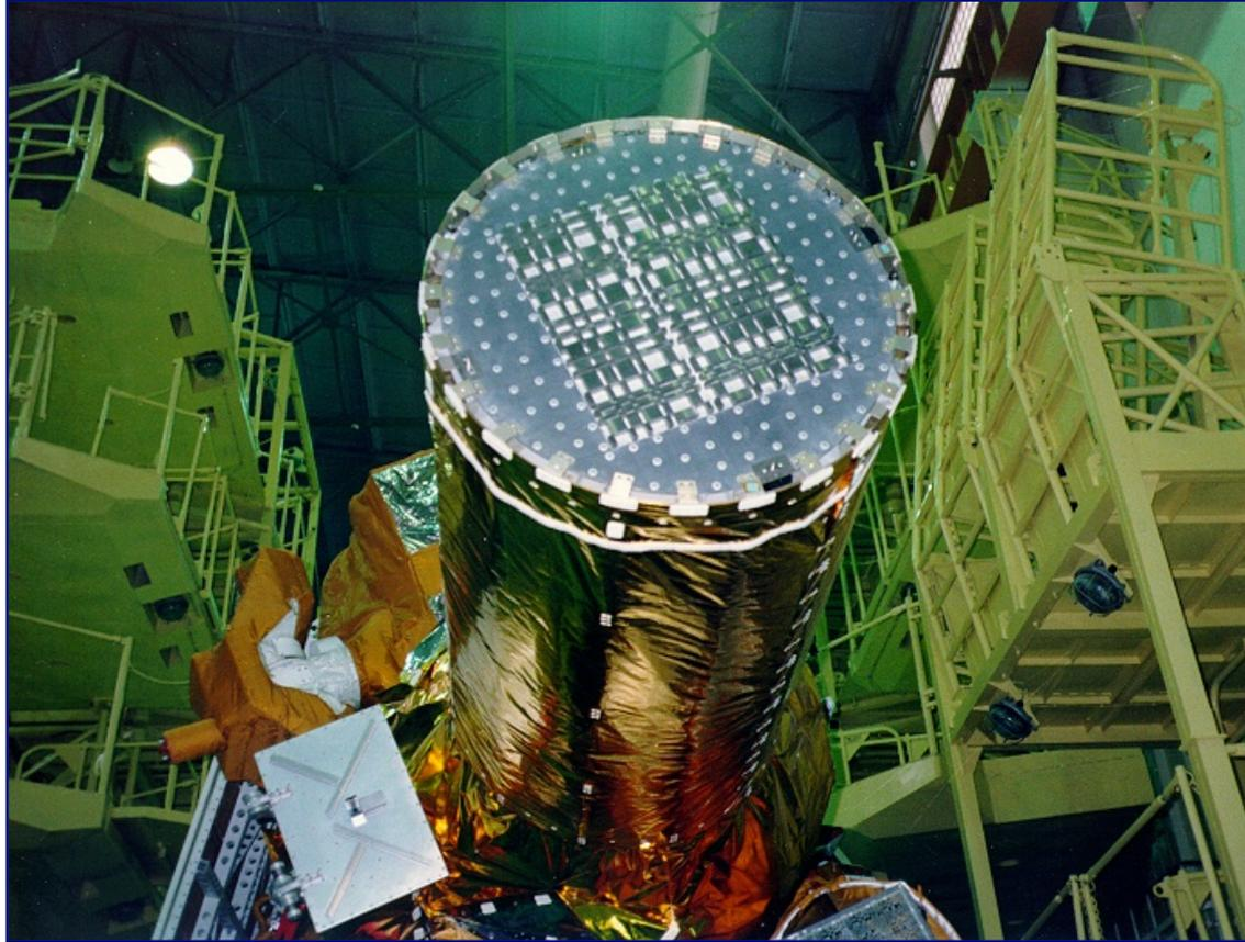
First space coded-mask telescope in operation from 1990 to 1997
